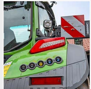
Push buttons operate the linkage – not very intuitive.
