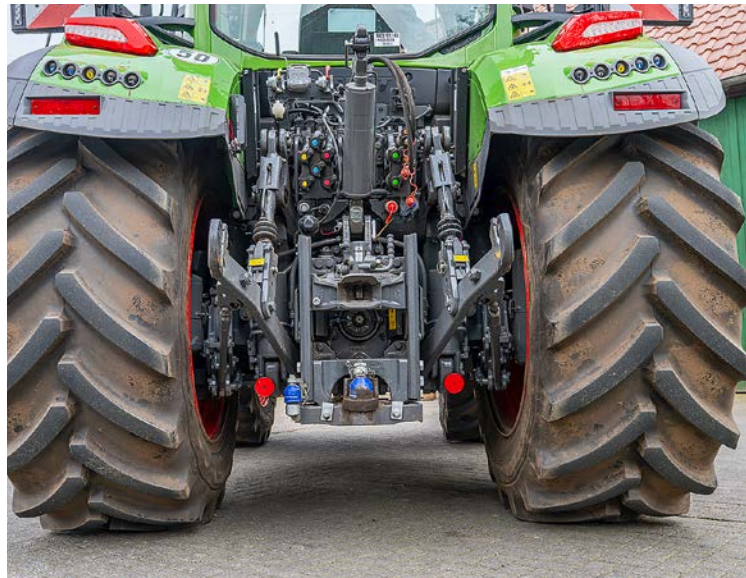
The rear: Powerful lift performance, and overall the back-end is well laid out. UK tractors get a Bennett pick-up hitch.
